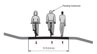
Photo 9.3: Cross-section of a shared-use path
