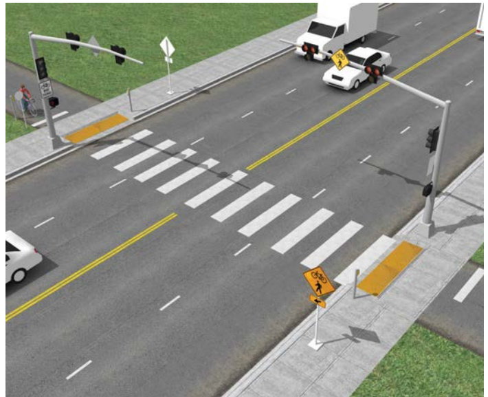
Photo 9.8: Mid-block crossing with HAWK signal
